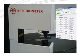
Measurement of light spectrum by transmission through the lens and/or reflection on its surfaces.
